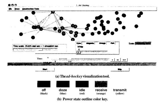
**Figure 18:** *Ad-hockey* with interface power state indication.
