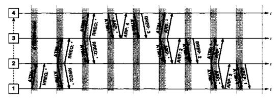
**Figure** 7: Route Discovery using IBSS power management.
