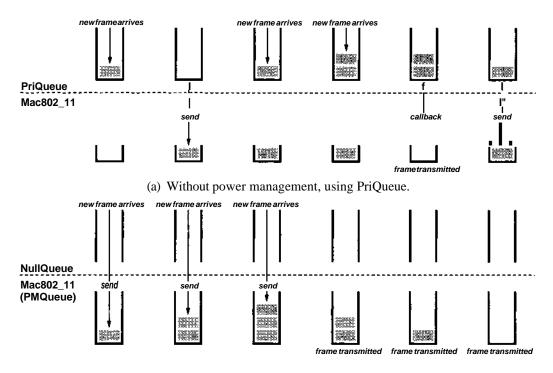
(b) With power management, using NullQueue and PMQueue in the 802.11 layer.
