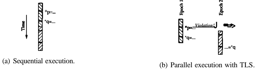
Figure 2: How TLS ensures that all reads and writes occur in the original sequential order.
