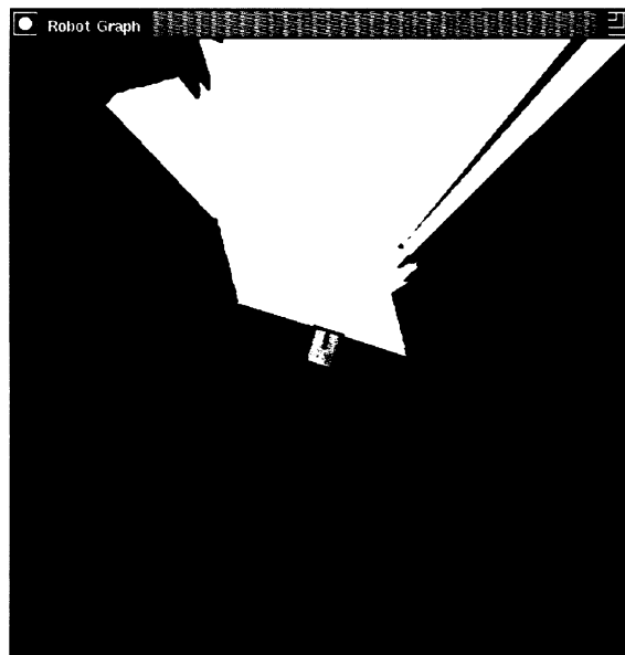
Figure 6: Range readings produced by laser range finders in a mobile robot Nomad XR4000. The robot is shown in the center. An occluded region is colored in light blue.
