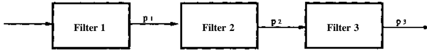
Figure 2: Searchlet Evaluation. The filters are applied, in sequence, to each object in the collection. The order of evaluation is chosen by the Diamond run-time environment. In the ordering above, Filter 1 is evaluated first, and passes p_1 of the objects to which it is applied. Filter 2 is evaluated next, passing p_2 of the objects passed by Filter 1; similarly, Filter 3 executes last, with a conditional pass rate of p_3 .
