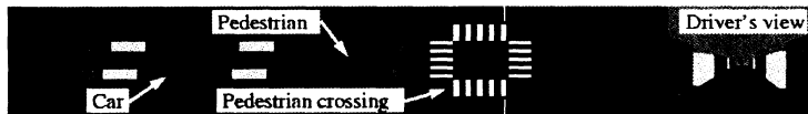
Figure 2: This scene consisting of a drivable area, non-drivable areas (sidewalk, grass), obstacles (parked cars), and a moving object (pedestrian).
