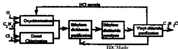
Figure 1: Principal steps in the vinyl chloride process
