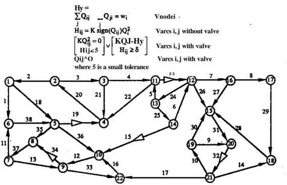
Fig.4. Pipeline example with five check valves.
