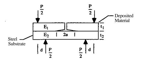
Figure 2. The Bimaterial Specimen
