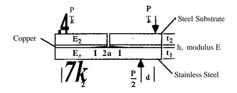
Figure 7. Three Layer Specimen for Stainless Steel Dripped on Copper
