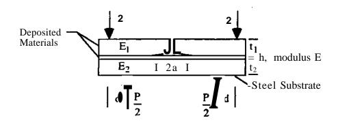
Figure 3. The Three Layer Specimen
