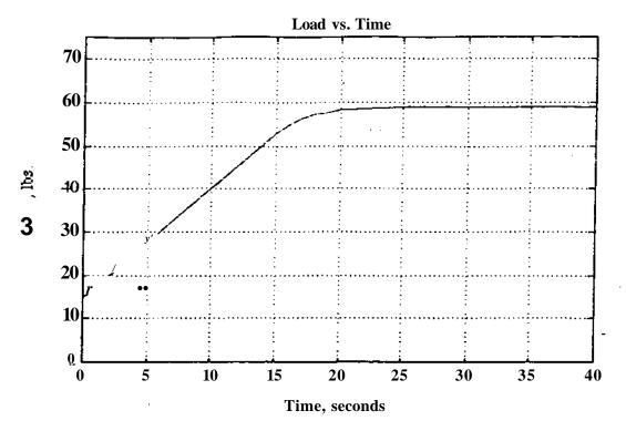
Figure 6. Load vs. Time for NiAl Sprayed on Carbon Steel
