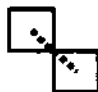
Figure 10: A "diagonal" edge is introduced in the Voronoi diagram (shown dotted) to reflect 8-connectivity
