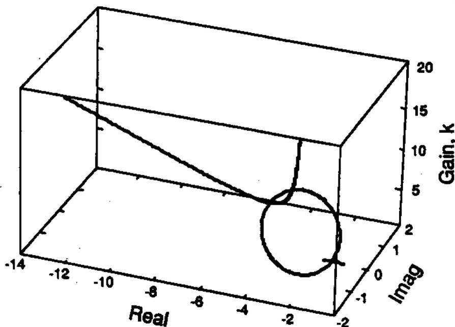
Figure 5. Three Dimensional Evans Root Locus Diagram of Equation (1).
