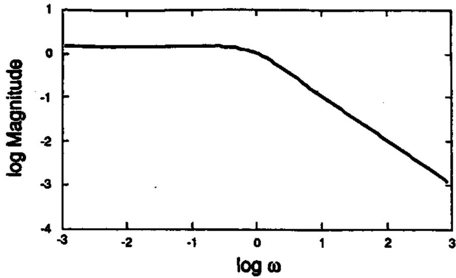
Figure 8a. The **Bode Magnitude Plot** of Equation (1).
