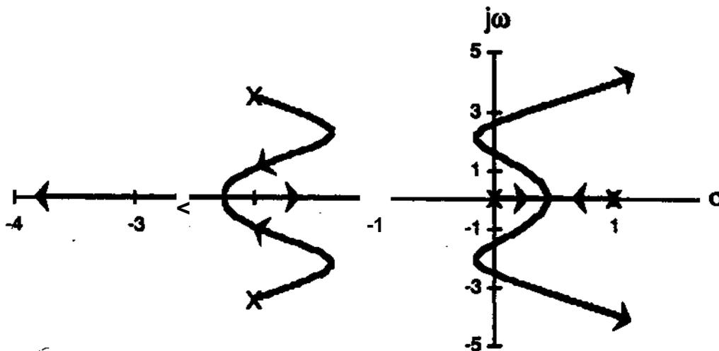
Figure 11. Root Locus for System Given by Equation (14).
