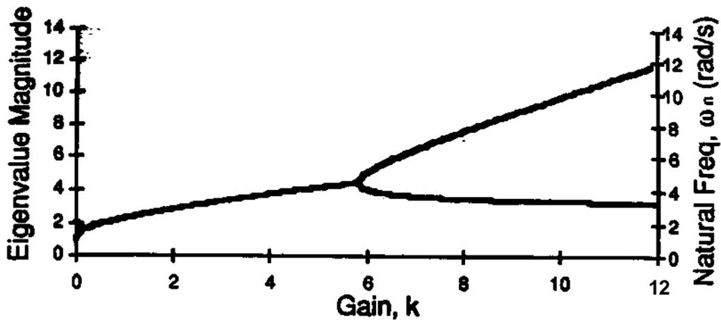
Figure 9a. The Variable Gain Magnitude Plot of Equation (3).
