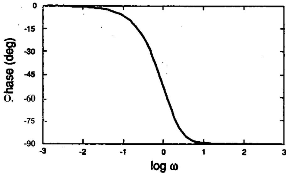
Figure 8b. The Bode Phase Plot of Equation (1).
