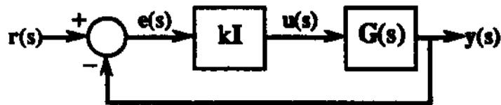
Figure 14. Closed-Loop MIMO Negative Feedback Configuration.
