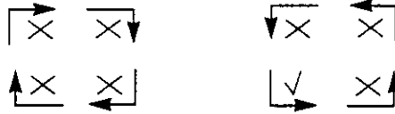
Figure 6: The corner-turns used by the restrictive route Y then route X router
