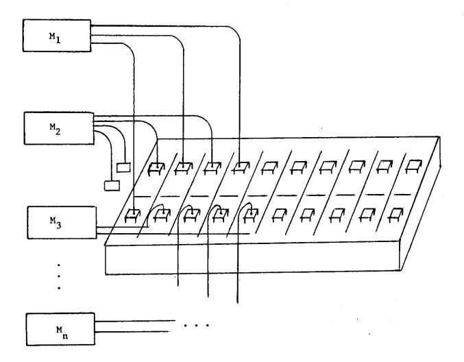
The use of the system is best illustrated by a simple example. Suppose one wished to construct a program to read text from a paper-tape reader and print it on the teletype. Modules exist for reading (characters) from the paper tape reader (PTREAD) and writing (characters) on the teletype (TIWRIT) -- so they can be interconnected as follows:
