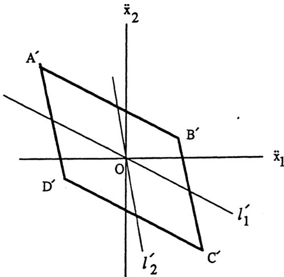
Figure 5: Image set of the linear mapping of a two degree-of-freedom planar manipulator
