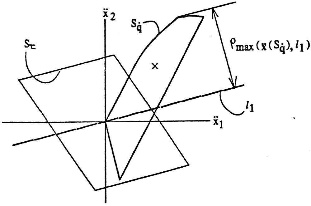
Figure 13: Maximum distance from reference line  $l_1$  to a point on the set  $S_q$
