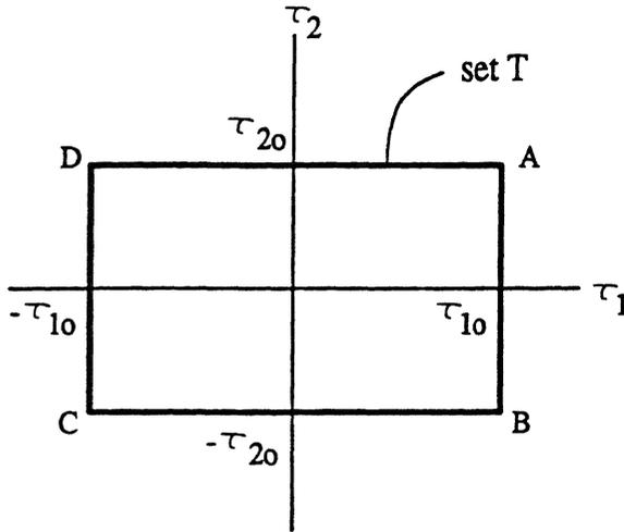
Figure 3: Set of the actuator torques of a two degree-of-freedom manipulator
