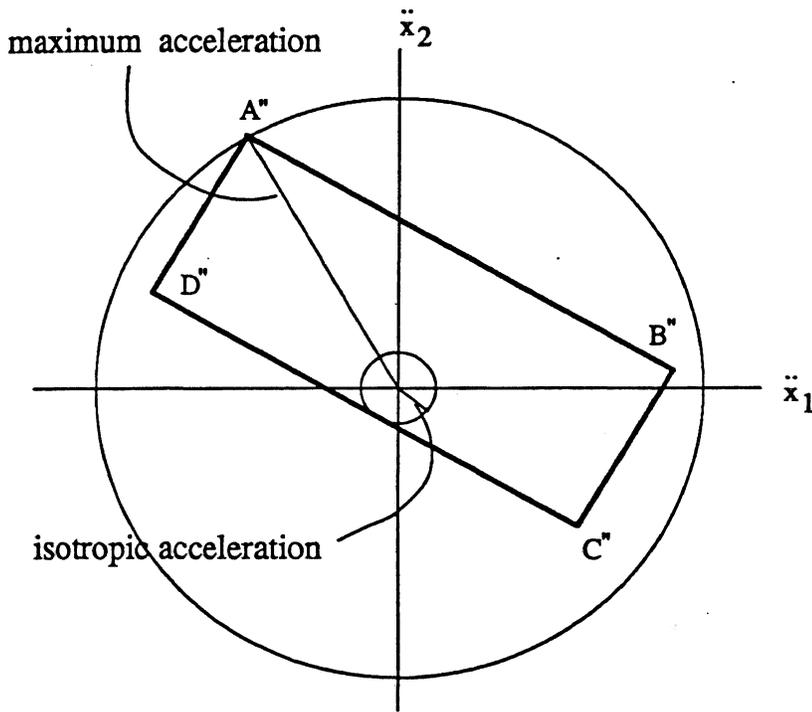
Figure 15: Characterization of the state acceleration set of a two degree-of-freedom manipulator
