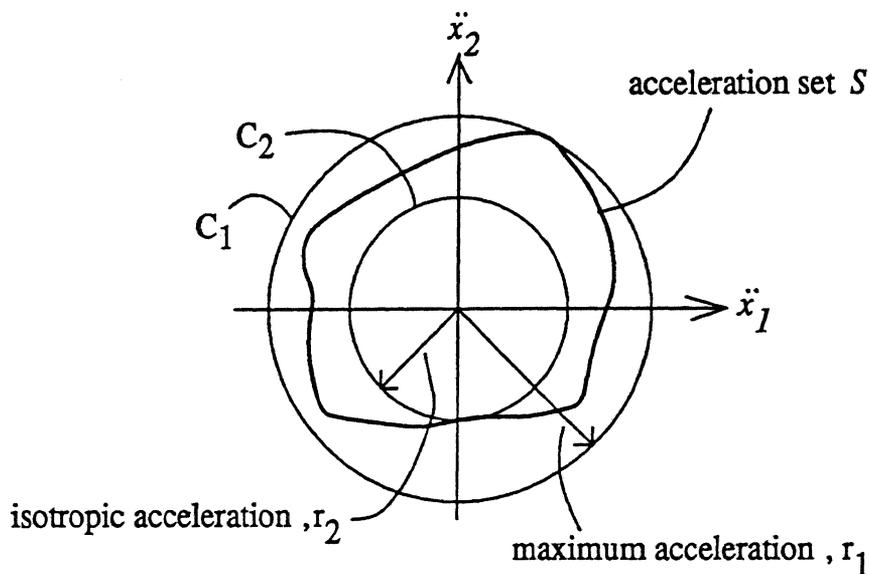
Figure 4: Characterization of an acceleration set in the acceleration plane
