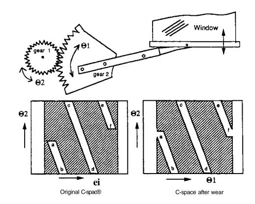
Figure 4-2: Example 2 : Window Regulator Mechanism
