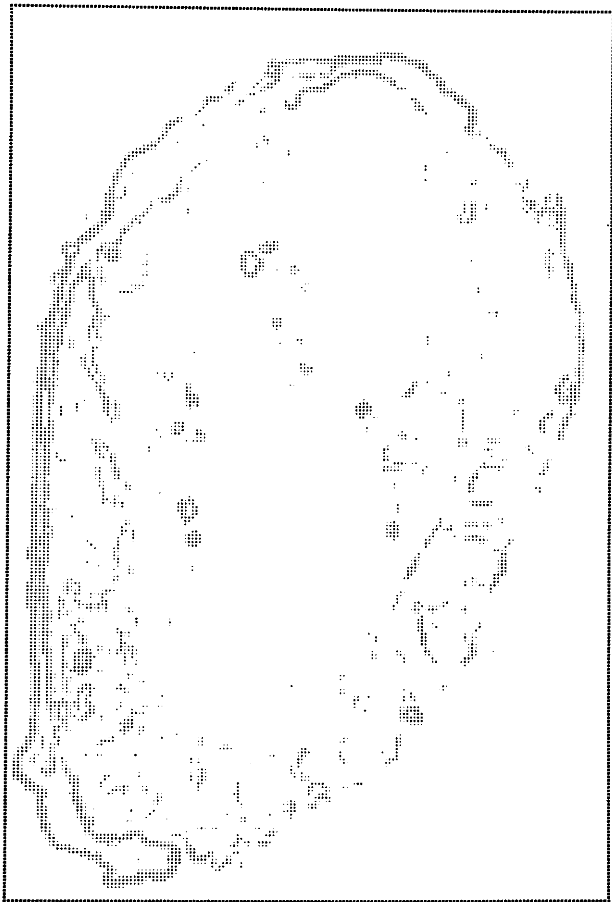
Figure 12-C. Attempt at edge detection of all interesting dendritic profiles and landmarks by applying a difference operator to the image in figure 10A; note that many undesired regions ("noise") also appearing the output.
