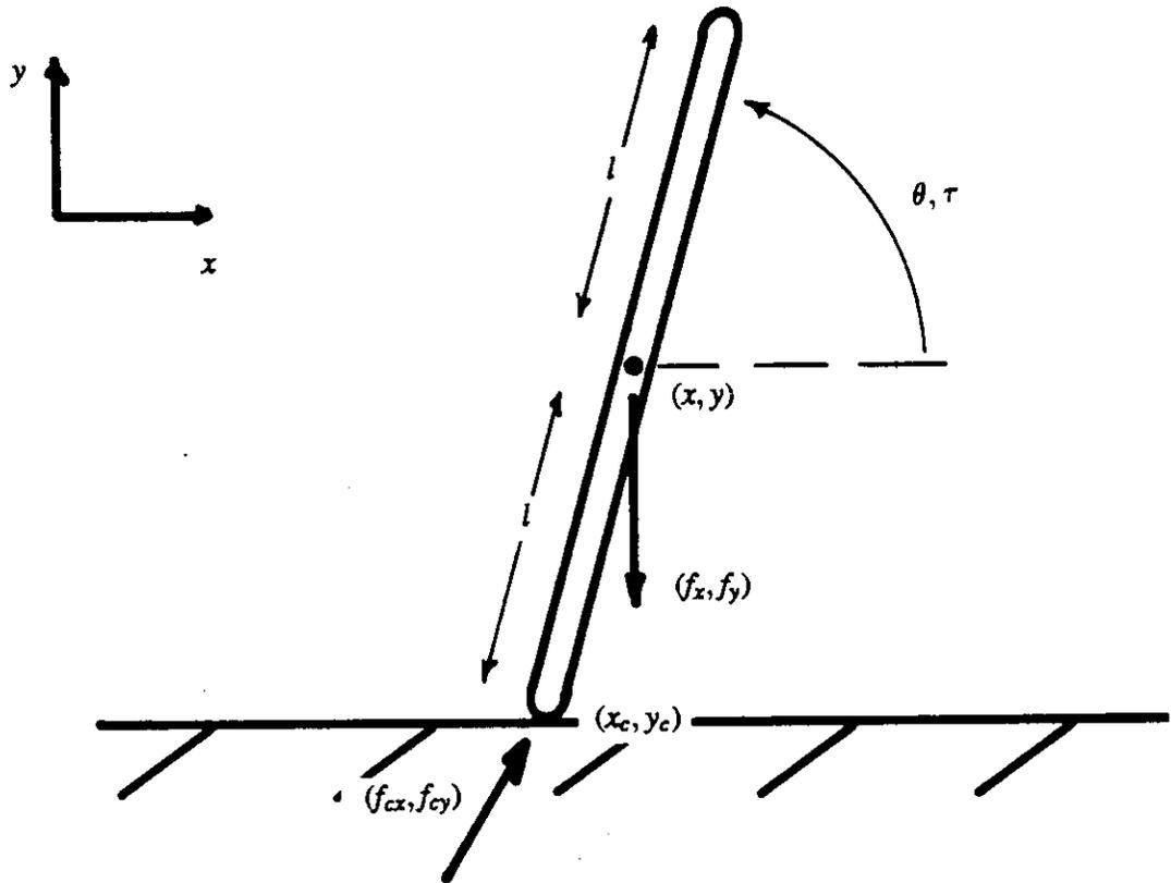
Figure 1: A rigid rod on a frictional surface.
