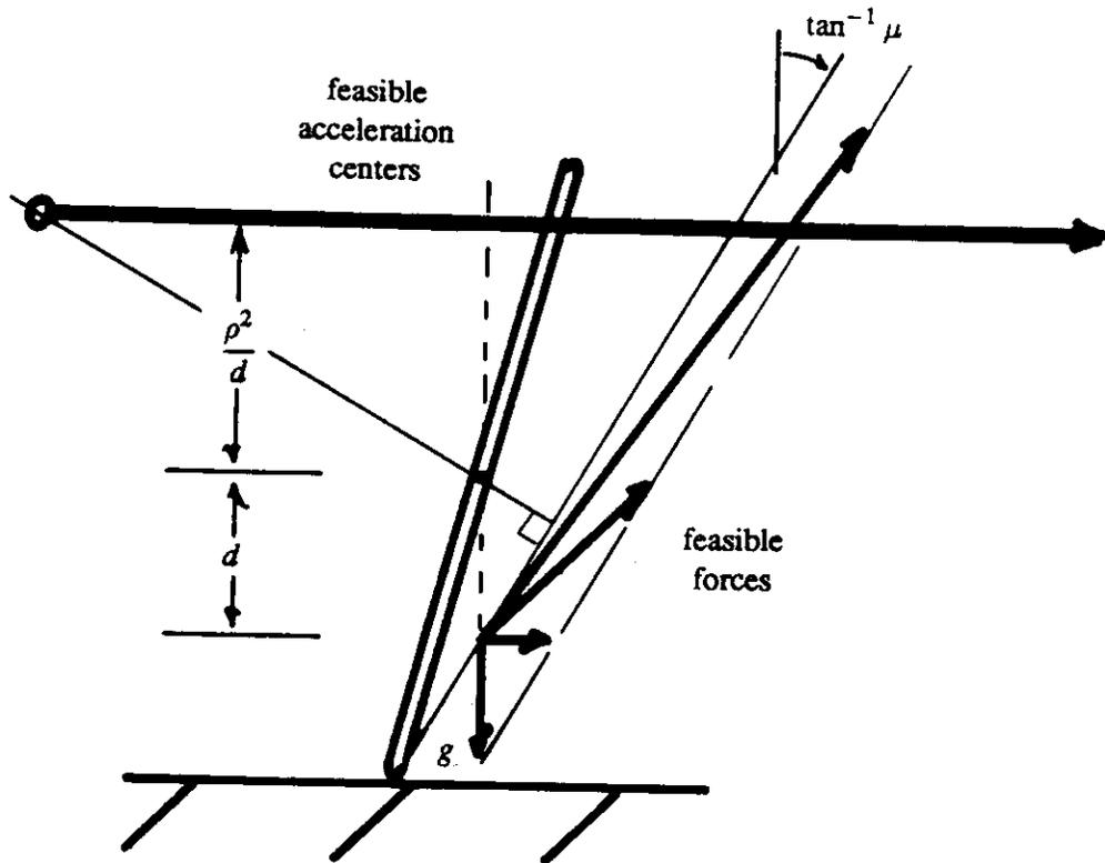
Figure 3: The locus of feasible acceleration centers.
