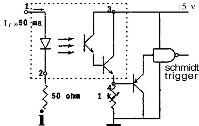
Figure 2: Transmitter-receiver pair and detection circuit
