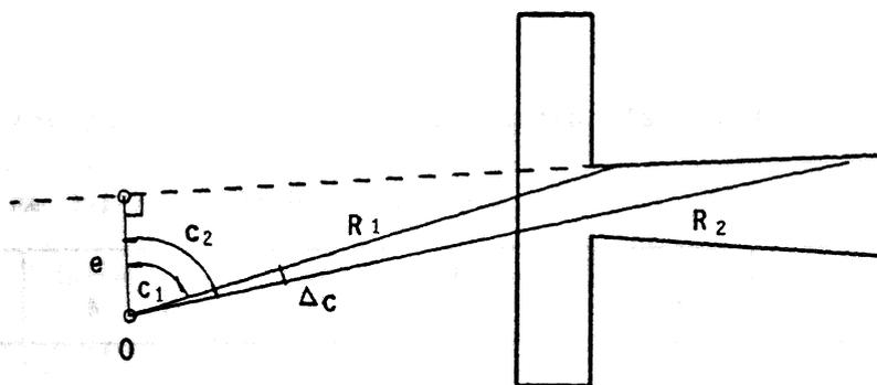
Figure 5: Error caused by inexact placement of the target
