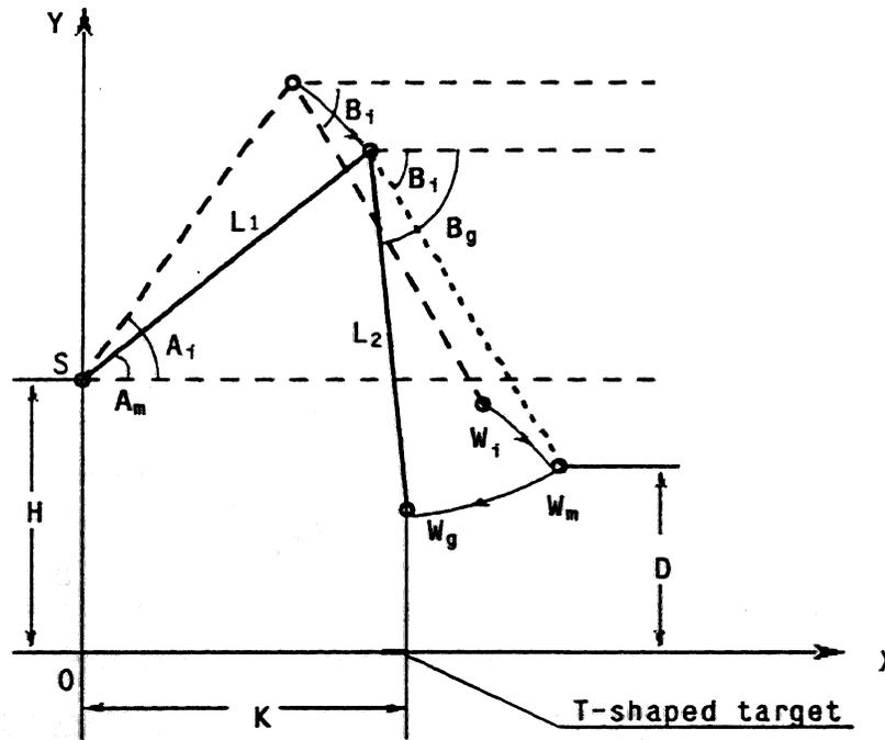
Figure 3: Steps 1 (shoulder-forward) and 2 (elbow-forward)
