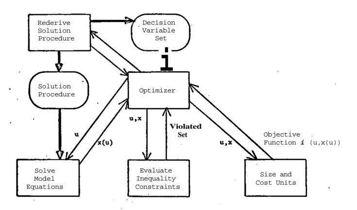
Fig. 1. Structure of an Optimizing System.
