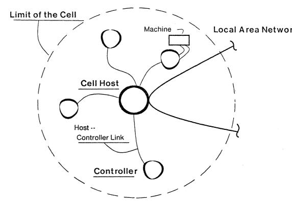
Figure 2-2: The Machining Cell Communication Topology
