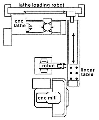
Figure 3-2: Machining Cell Layout -- First Arrangement
