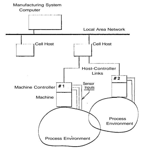
Figure 2-1: Hierarchical System Design
