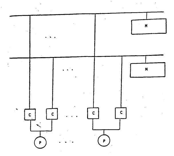
Figure 7-1: Multiple Shared Bus Cached Based Parallel Processor
