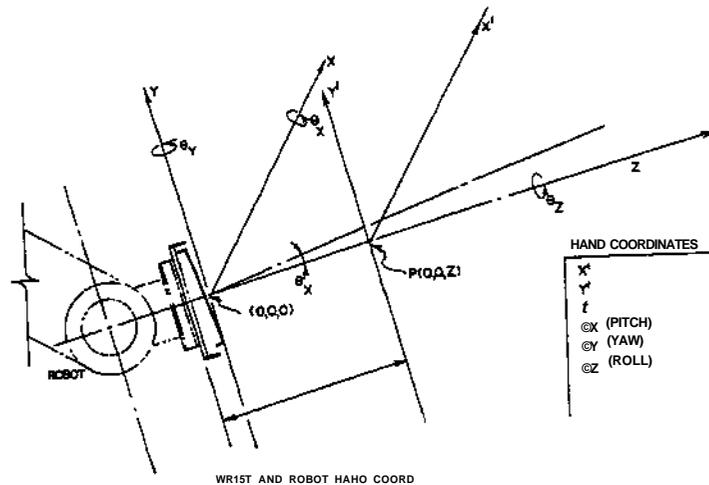
Figure 8: Coordinate system for robot control
