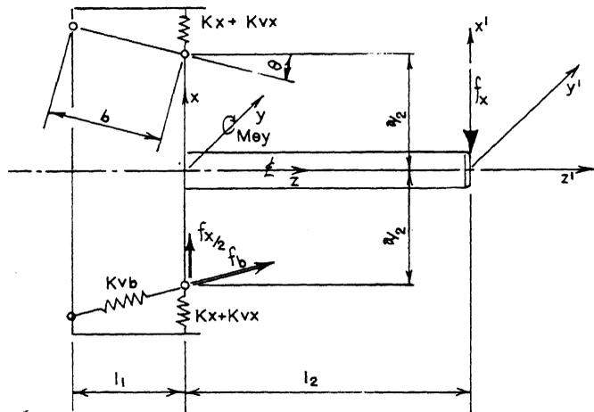
Figure 6: Spring representation of new wrist
